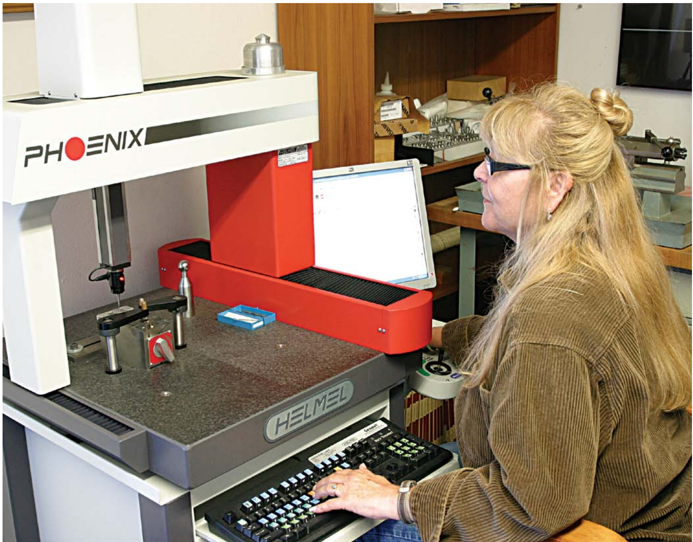
Milo Engineering quality inspector, Linda Couvrey, checks a miniature part on the company's Helmel Phoenix CMM. The CMM offers a 12" x 12" x 10" work envelope. Milo vp Ray Hofer says the machine was easy to learn and has performed flawlessly since he purchased it in August 2009. The automated system outputs full documentation for all inspections. it is used to check 15 to 60 critical dimensions.
