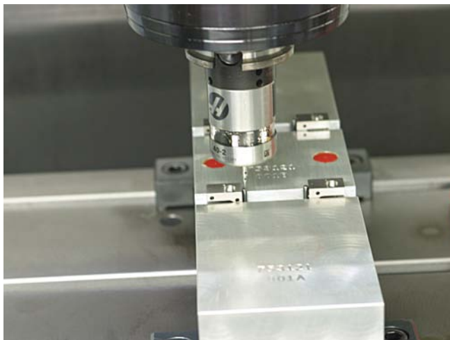
Renishaw touch probe at work on a Haas vmc.
