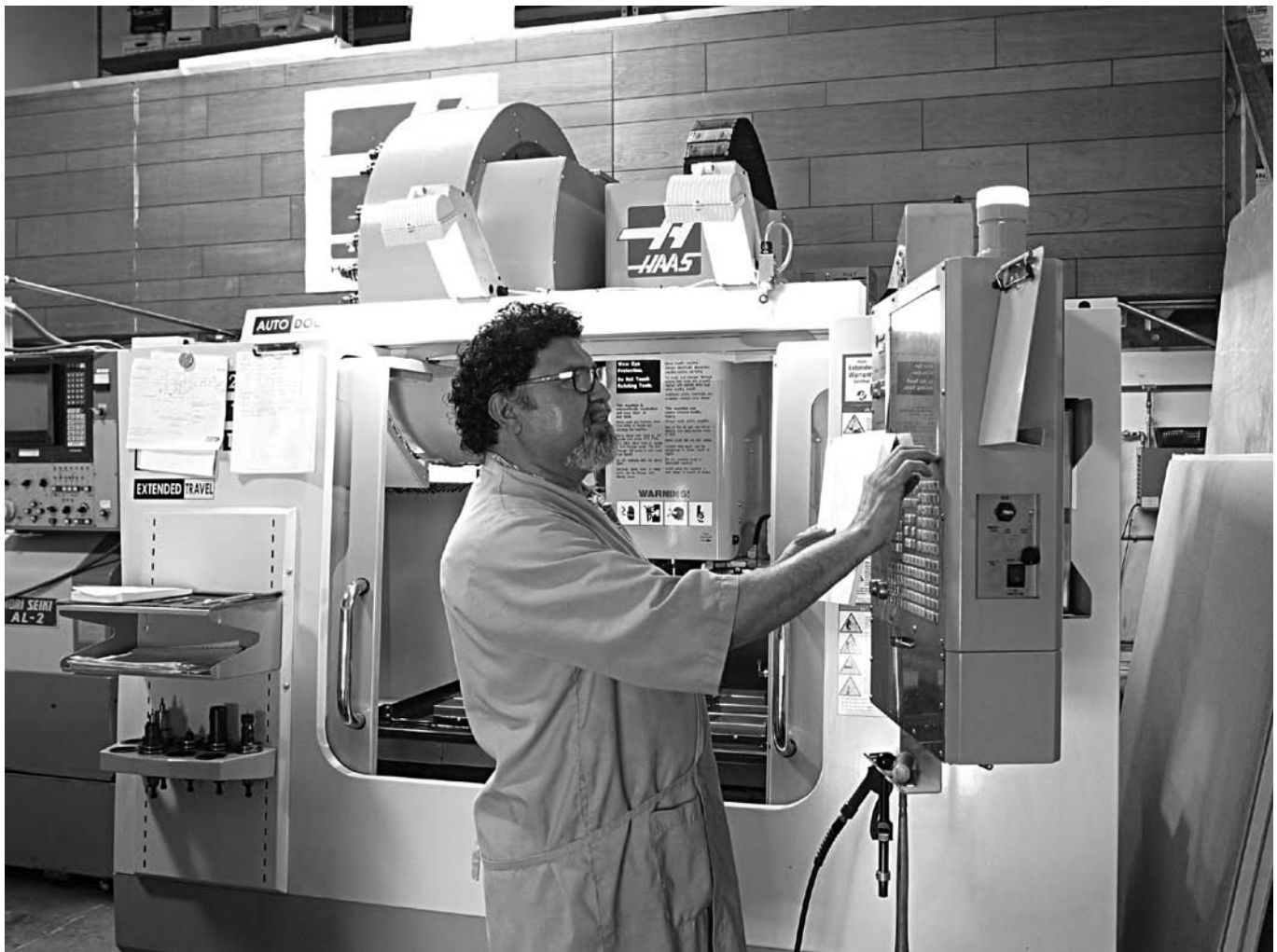
CNC operator Norman Villegas sets up a Haas VF2-YT equipped with a Renishaw touch probe system. Part to be produced is a Kovar gyro for the Global Hawk program.
